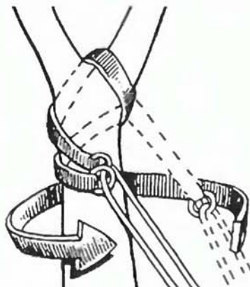
The false crotch is also a “moving crotch” that follows the climber’s movements in the tree while providing consistent friction.
