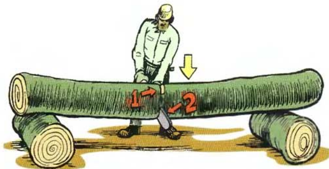
FIGURE 7.17 If there is upward pressure on the limb, start with a small top cut and finish from below.
