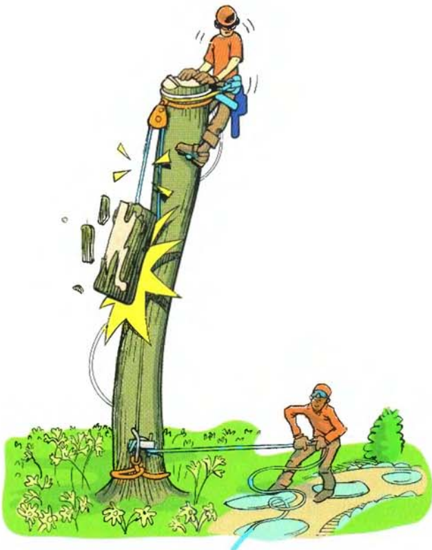
FIGURE 6.4 Shock-loading occurs when a dynamic, sudden force is placed on a rope or rigging apparatus when a moving load/piece is stopped.
