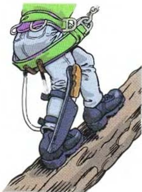
FIGURE 4.28 Most climbers climb with their handsaw and scabbard (sheath for the handsaw).
