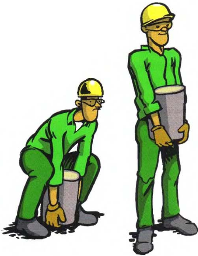
FIGURE 7.20 Proper lifting technique can help prevent back injuries.
