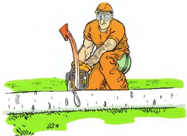
FIGURE 7.15 When bucking a log, keep your body away from the chain-saw path. Leg protection is required by ANSI.
