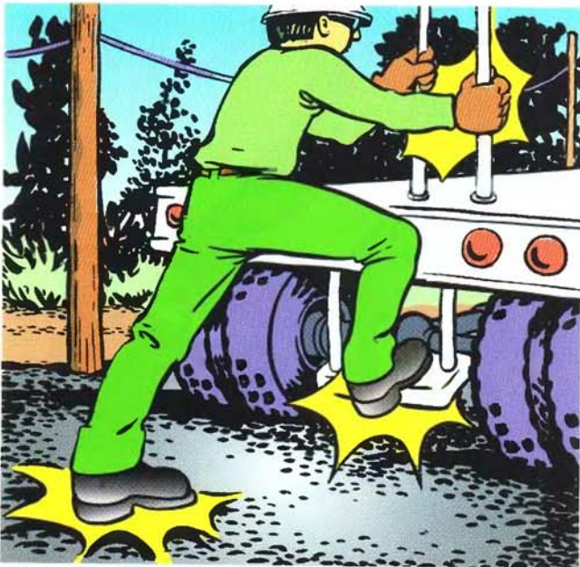
FIGURE 2.15 A climber can be electrocuted as a result of indirect contact with an energized conductor.
