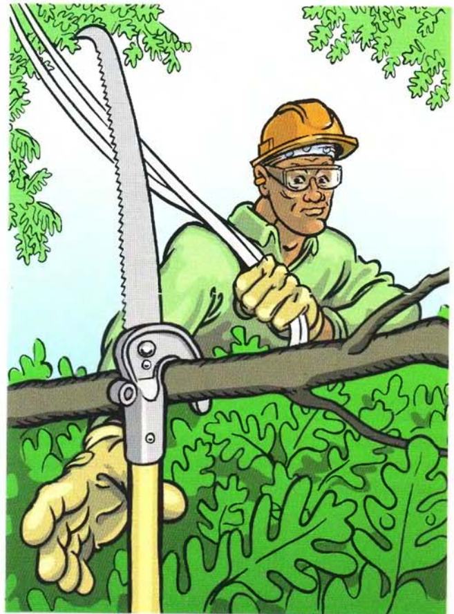
FIGURE 4.29 If pole pruners or pole saws are used in the tree, they should be hung vertically in the tree when not in use. They should be hung in such a way that the sharp edge is away from the worker and so that they will not accidentally dislodge.
