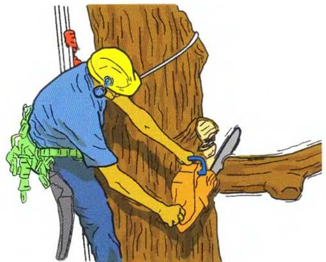
FIGURE 6.24 When using a chain saw to make a drop cut, climbers should form the top cut directly above the undercut to avoid getting the bar stuck in the kerf of the cut as the limb breaks free.
