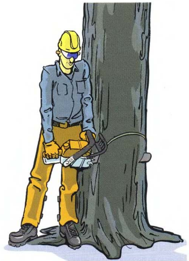
FIGURE 7.10 The worker can position himself to cut the notch facing the desired direction of fall.
