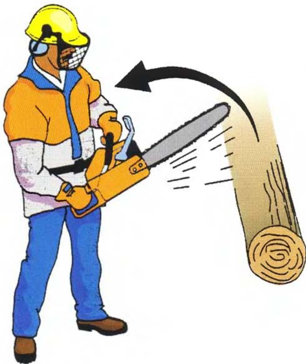
FIGURE 2.21 Kickback results when the upper tip of the guide bar contacts an object.
