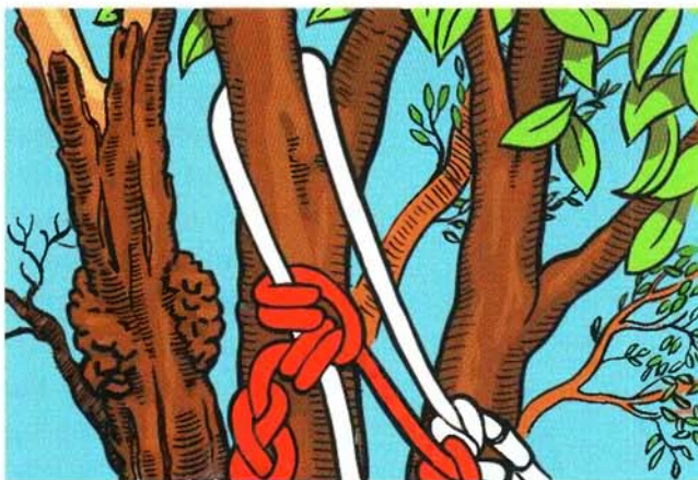
FIGURE 4.20 Choice of where to place the line is important. Choose a sturdy limb and lateral branch. Tie in around the parent limb or trunk and over the lateral limb.
