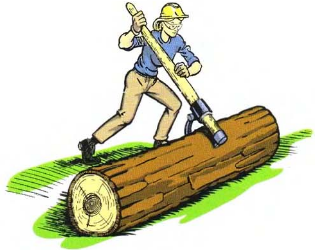
FIGURE 7.19 Safe and proper use of tools, such as the cant hook and peavey, can eliminate many accidents.
