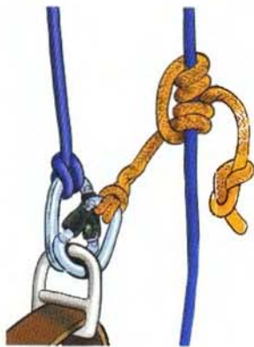
FIGURE 4.22 A split-tail is a separate, short length of rope used to tie the friction hitch in a climbing system.
