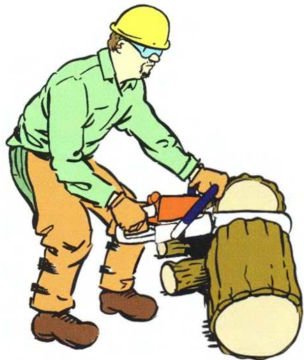
FIGURE 2.17 The chain saw should be firmly gripped with both hands. Keeping the left arm straight helps to control the saw.
