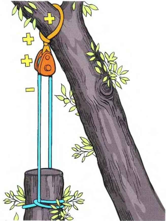
FIGURE 6.8 Arborists generally design rigging systems so that the rigging line (load line) is the weakest link in the system.
