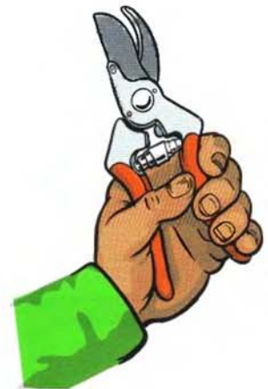
FIGURE 5.1 Hand pruning shears (secateurs) work best with two bypass blades. Avoid the blade and anvil design, which can damage stem tissues.
