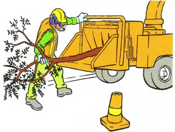
FIGURE 2.25 Brush should always be fed from the side, and the worker feeding the brush should move away after the brush is fed. The larger butt end of each branch should be fed in first.
