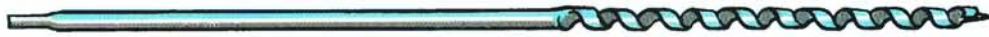
FIGURE 8.17 A ship auger is used to pre-drill the holes for cable hardware installation.
