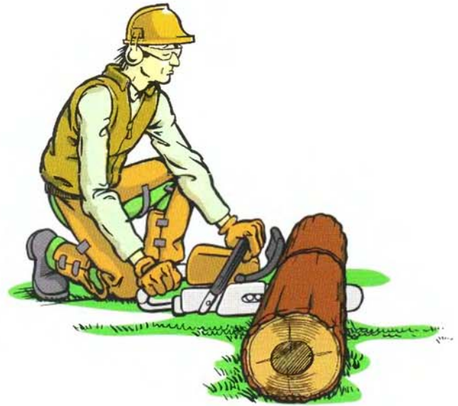
FIGURE 7.14 Position yourself so as to avoid grounding the saw.
