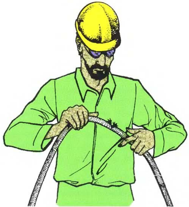
FIGURE 4.4 Climbers should always inspect their climbing line before each use. Retire ropes with excessive wear or cuts.
