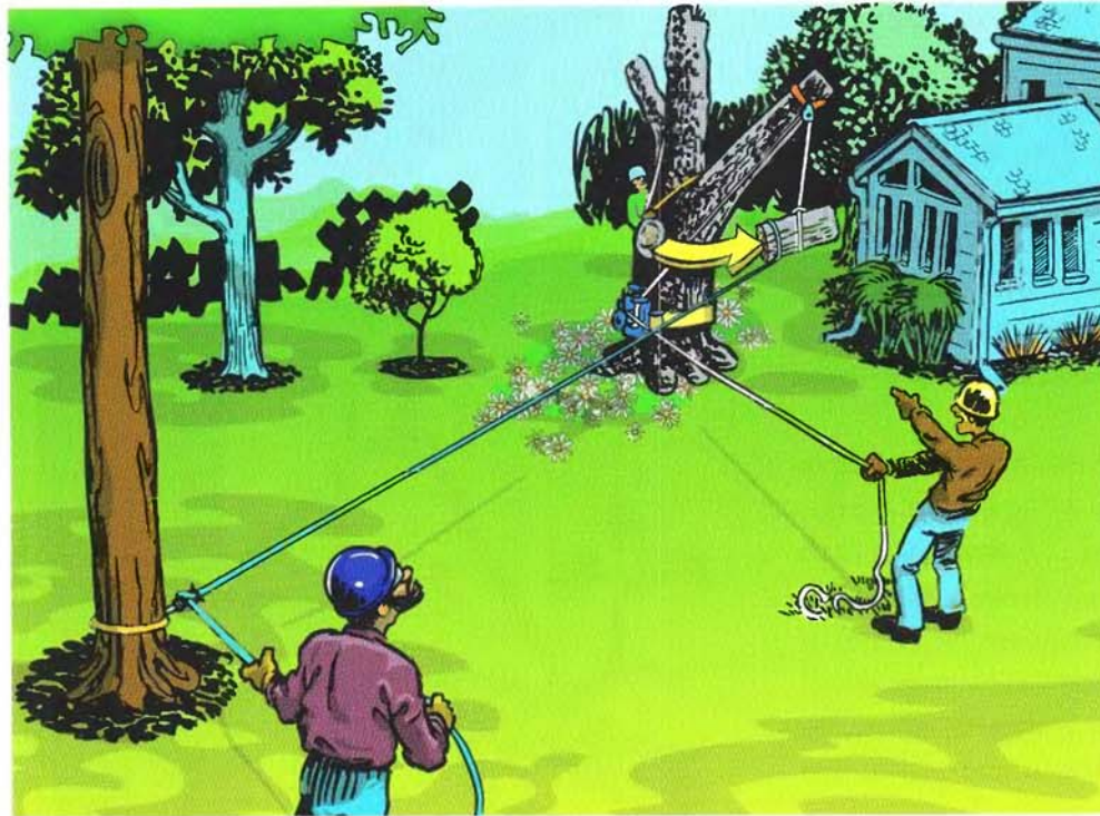
FIGURE 6.22 A tagline may be attached to help the ground worker control the piece being removed.
