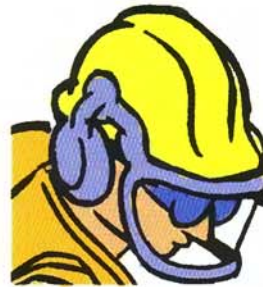
FIGURE 2.6 Some hard hats have integrated ear muffs, although earplugs may also be worn.
