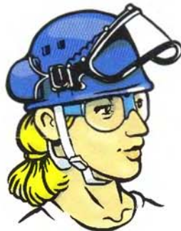
FIGURE 2.4 A face shield provides added protection against flying debris, but it is not a substitute for eye protection.
