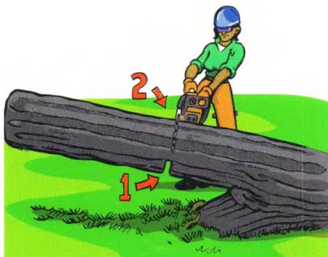
FIGURE 7.18 If the limb is under downward pressure, start with a small undercut, then finish from the top.
