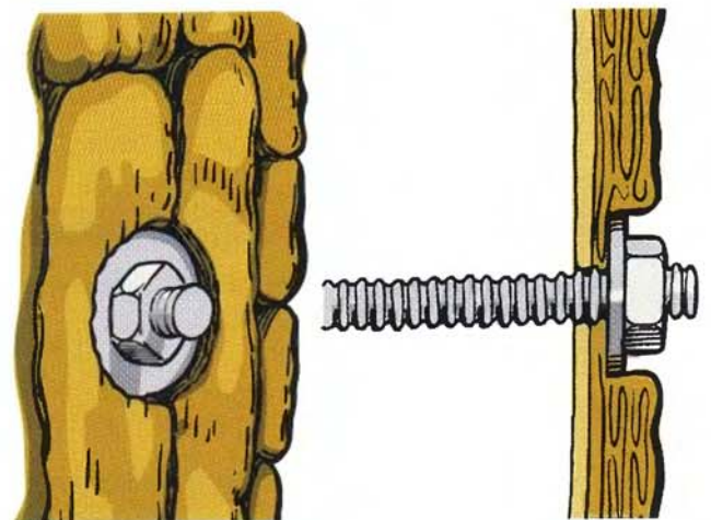
FIGURE 8.7 On most trees, seat the washer directly on the bark. On trees with very thick bark, countersink the washer to the sapwood.
