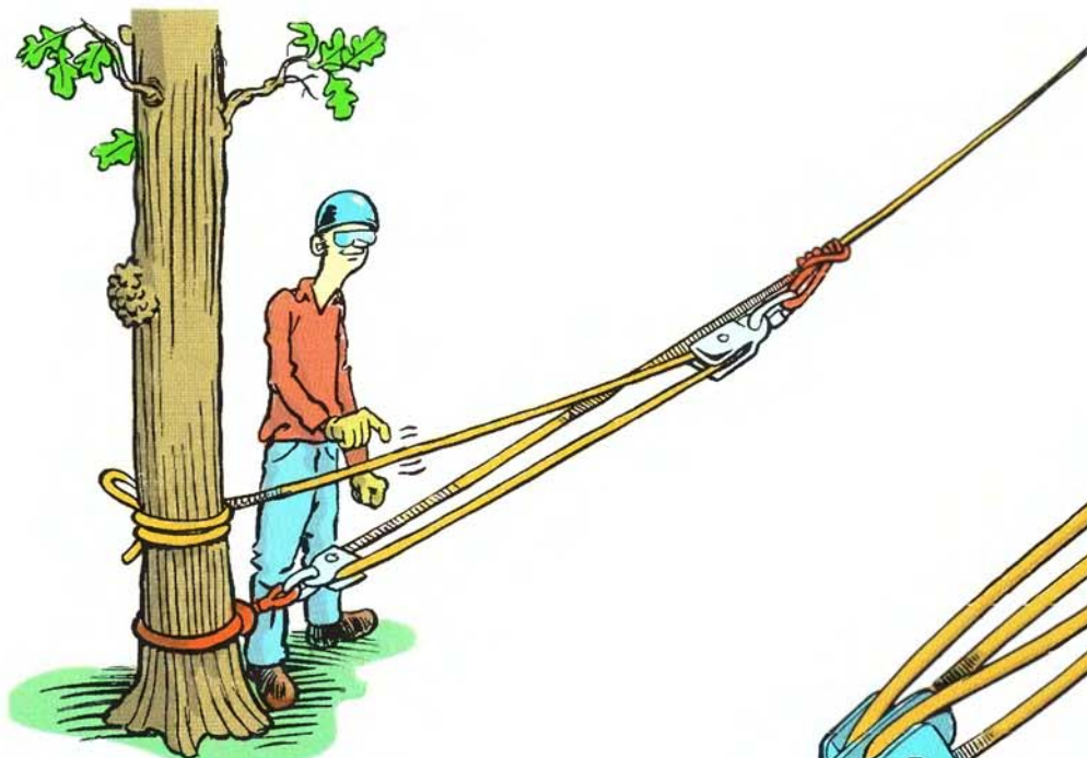
FIGURE 7.5 A pulley added to the system will reduce friction on the rope.
