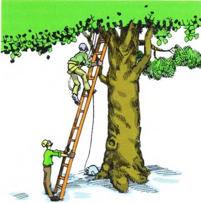
FIGURE 4.9 A second worker should always support the ladder while a climber ascends.
